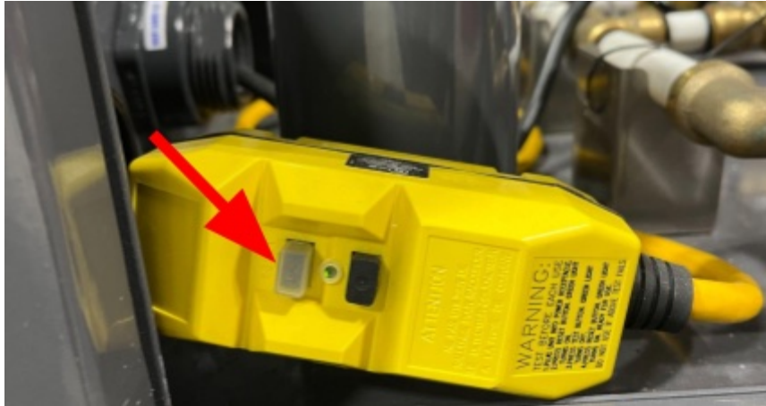
Figure 8) Turning on the GFCI Breaker
