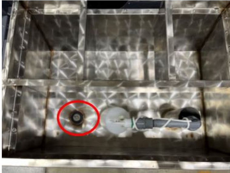
Figure 15) Drain Plug Location
