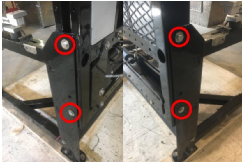
Figure 20) Loosen four bolts to raise/lower the front of SmartFeed
