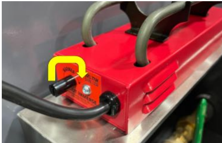
Figure 7) Main Heater Adjustment
