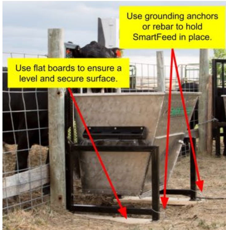
Figure 2) SmartFeed Orientation and Mounting Reference
