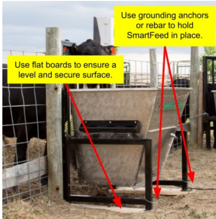
Figure 2) SmartFeed Orientation and Mounting Reference
